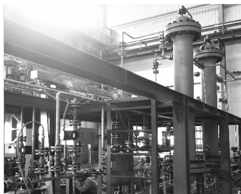
Fig. 18 A pilot setup of PTFE membrane contactor system
